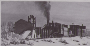
Locomotive 268 with wedge snowplow 09271, flanger OJ, cabooses 0524 and 0588 on a snow plow run from Gunnison to Sapinero, March 11, 1952. (Photograph by Robert W. Richardson, Colorado Railroad Museum)
