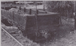
Ex-D&RGW drop bottom gondola number 769 in service on the Cumbres & Toltec Scenic Railroad at Chama, New Mexico, March 1972. Drop bottom gondolas were often used to haul cinders removed from the locomotives. They were spotted on a depressed track (as shown here) so that the cinders could be shoveled from the locomotive into the car. (photograph by Jerry B. Day)
