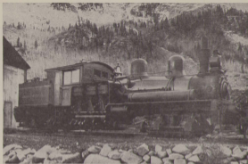
Shay mechanism is aptly shown in this McClure photo. Note stove pipe extension in stack. Western Collection Denver Public Library.
