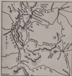
Extension of the Argentine Central through the Argentine Tunnel and connection with the Colorado and Southern or Rio Grande at Keystone would have shortened Denver-Leadville distance to 122 miles, vis-a-vis 276 miles by Rio Grande standard gauge, 189 miles via Como and Boreas Pass on the South Park.
